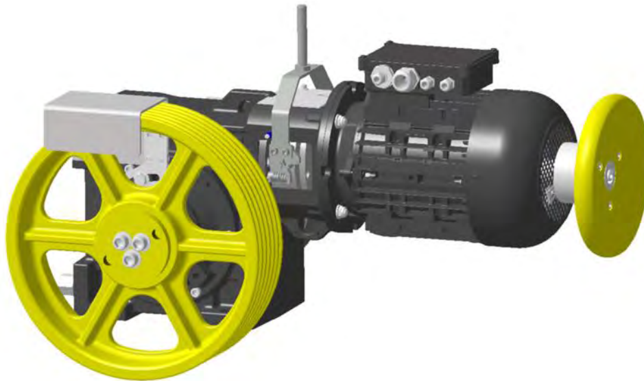
Fig. 2-4: TW45C machine - version for installation site – machine room with horizontal rope departure direction – SA1 (shown: traction sheave position - left / motor position - horizontal)
