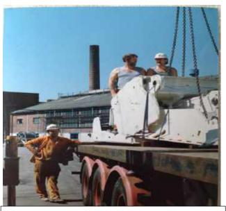
Delivering Gullick Dobson roof supports to a coal mine
