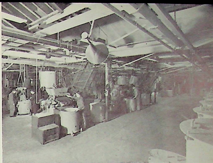
A line of refining mills in the Keystone Paint and Varnish Works
