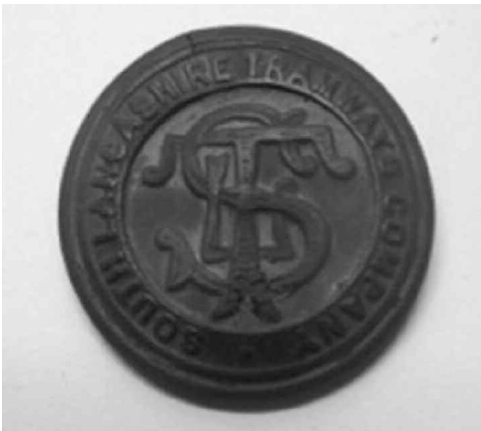
A die-formed three-piece South Lancashire Tramways Company uniform button with separate fitted wire shank, circular, hollow, convex front, concave back, crimped joint, SLT monogram, around which the inscription, SOUTH LANCASHIRE TRAMWAYS COMPANY.
