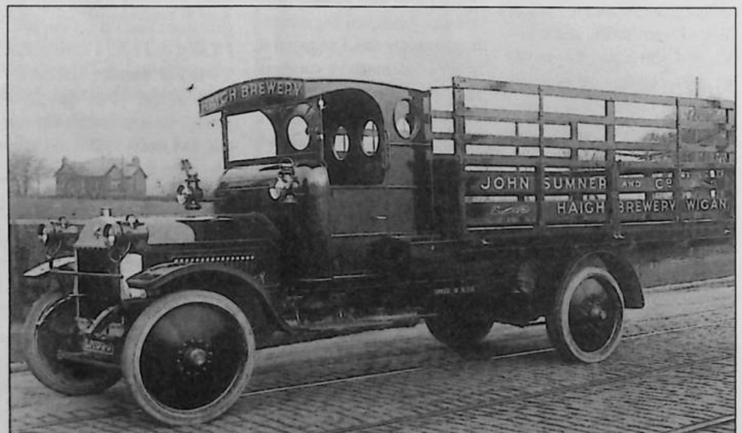
A 5-6 ton 12 m.p.h. Leyland solid-tyred wagon. Four such vehicles were used by Sumner's Haigh Brewery
