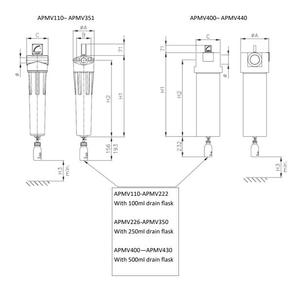
Aluminium range with threaded connections (as per ISO 7/1, BS 21, manufactured according to the European Directive CE 97/23 – PED, where applicable.
