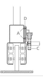
• Determine the installation position of the toothed rack on the gate.
