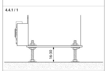
The height of the motor unit can be adjusted using the heavy-duty wall plugs.
