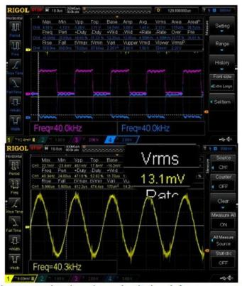
The transmitted and received signal frequency was  $40 \ kHz$ . The received signal  $V_{RMS} = 13.1 \ mV$ , which means that the "link budget" is:
