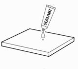
Fill the drilled holes with a good quality Sealant.
