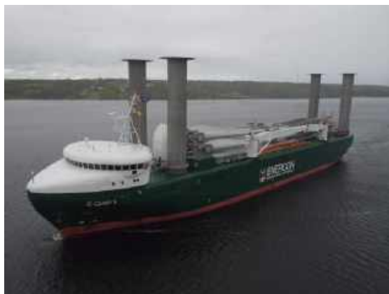
Flettner rotor on E Ship 1, source: IWSA
