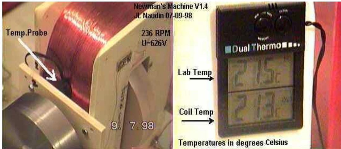
Figure 1: The temperature sensor and temperature readings Naudin recorded on his Newman Generator. Naudin's tests showed an endothermic electric effect or has he called it, 'a cooling effect'
