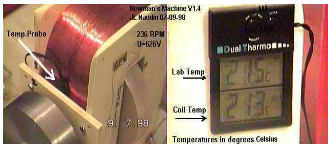
Figure 1: The temperature sensor and temperature readings Naudin recorded on his Newman Generator. Naudin's tests showed an endothermic electric effect or has he called it, 'a cooling effect'
