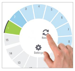
3 After the rack is rotated to the front, you can remove the rack. (The status light in the loading area blinks to indicate the location of the rotated rack).
