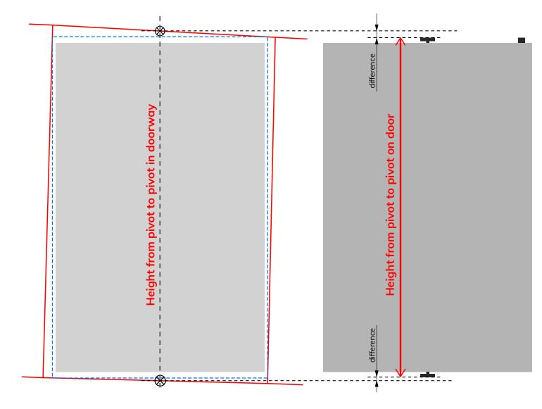
Check the pivot height of the door with the doorway measurements, and synchronize them if necessary.
