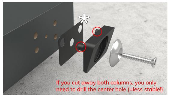
Mark and drill the holes for the 1-way part into the door leaf according to pattern below:
