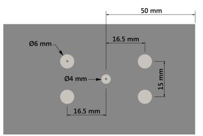
Install the optional 1-way under the magnet with the supplied screw.
