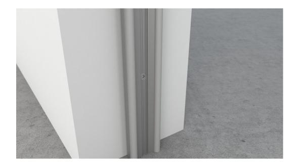
Use the supplied screws to install the profile to the wall.
