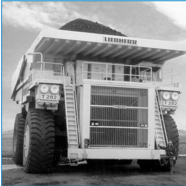
A huge double-unit SRG29 Donaclone™, our largest engine air cleaner, protects this haul truck under severely dusty operating conditions. The SRG29 Donaclone™ has 3 dust cups on the bottom of the unit.
