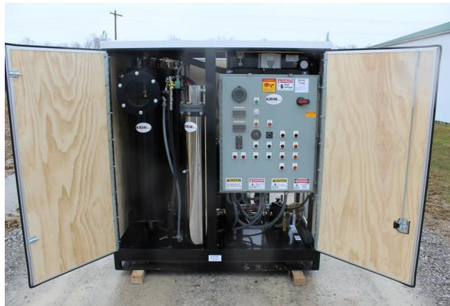
For Drying and/or De-Gassing substation transformers or tap changers WHILE the transformer is ENERGIZED.
