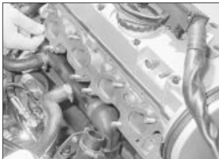
13.33 Fitting a new inlet manifold gasket
