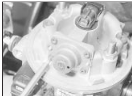
11.17a Undo the retaining screws ...
