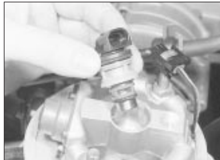
11.6c ... and remove the injector
