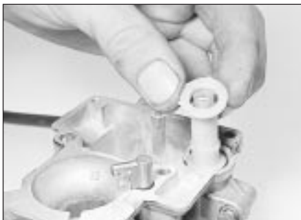
21.7a Removing the accelerator pump collar ...
