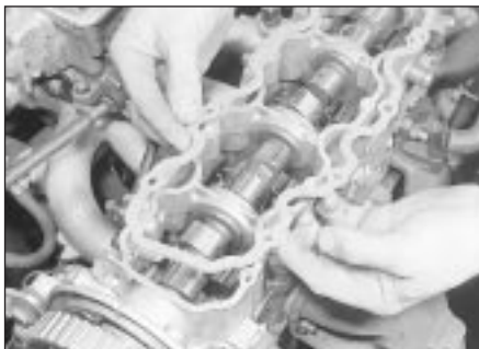
8.29a Fitting a new camshaft cover gasket
