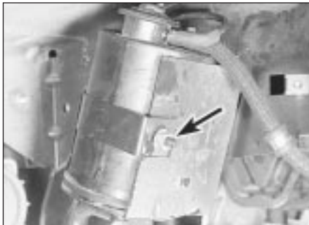
12.98a Canister clamp nut (arrowed)
