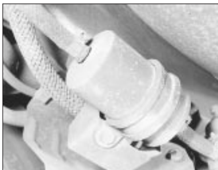
25.3 Fuel filter showing mounting and hose connections
