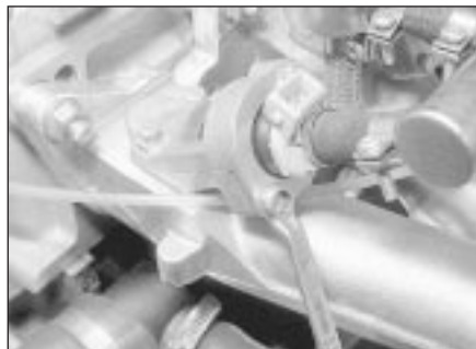
12.8 Undoing a fuel injector retaining bolt
