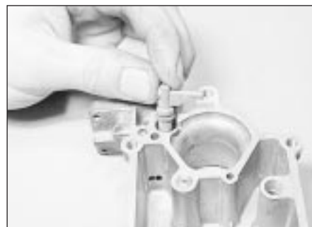
19.11 Removing the fuel discharge nozzle
