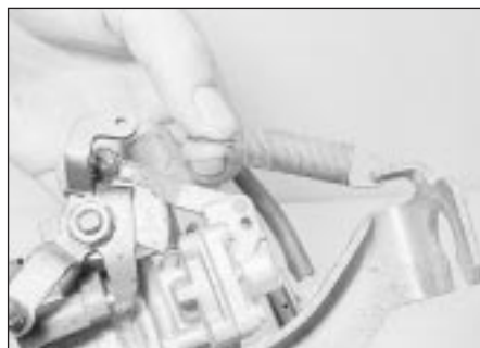
19.3 Removing the throttle return spring
