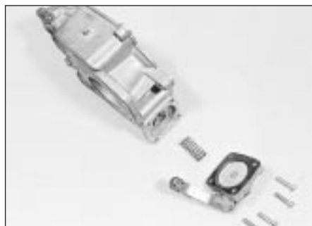
19.9 Accelerator pump components
