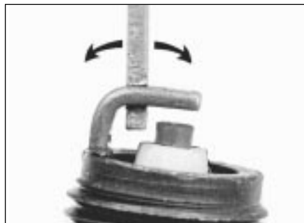
Adjusting spark plug gap
