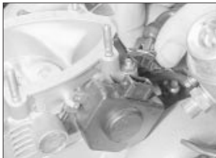
12.82 Disconnecting the throttle valve switch multi-plug
