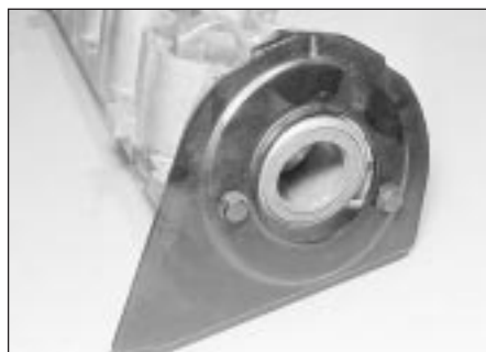
9.7 Camshaft belt cover backplate (1.3 litre engine shown)
