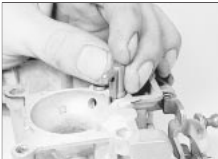
21.8 Removing the accelerator pump delivery tube
