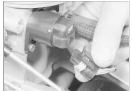
11.11a Detach the wiring connector ...
