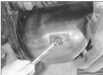
6.4 Removing the sump drain plug
