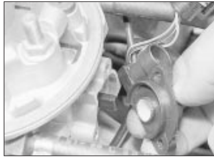
11.3b Throttle valve potentiometer removal
