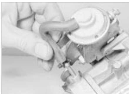
19.4 Disconnecting the vacuum hose
