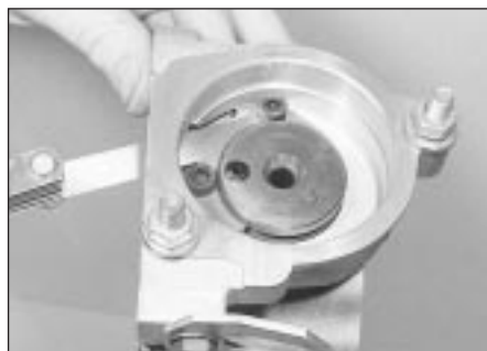
9.10 Checking the camshaft endfloat
