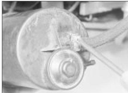
12.98b Disconnecting a hose from the canister
