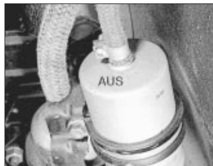
25.4 Fuel filter directional marking
