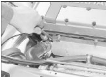
14.3 Removing an exhaust manifold heat shield bolt
