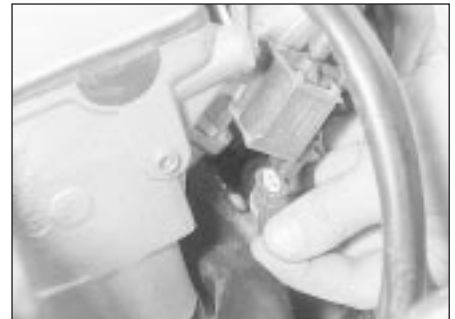
12.100 Disconnecting the vent valve multi-plug
