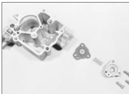
19.10 Enrichment valve components
