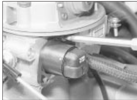
11.11b ... undo the retaining screws ...
