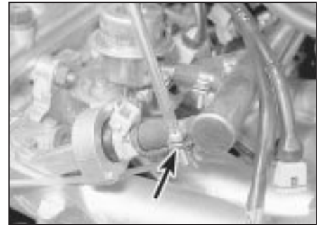
12.6 Slackening a fuel rail hose clamp
