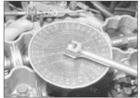
8.26b Using a marked card to measure angular rotation when tightening cylinder head bolts
