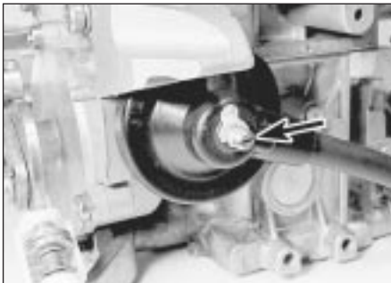
14.8a Choke valve gap adjustment screw (arrowed)
