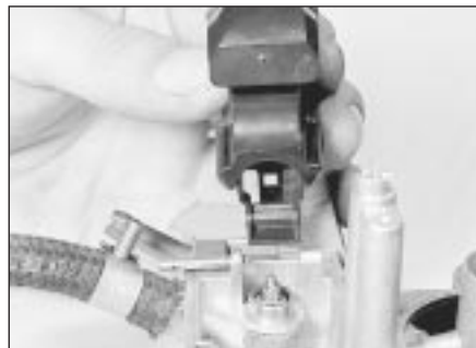
21.9a Removing the float ...
