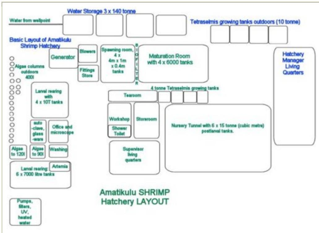
Hatchery layout plan allowing good biosecurity
