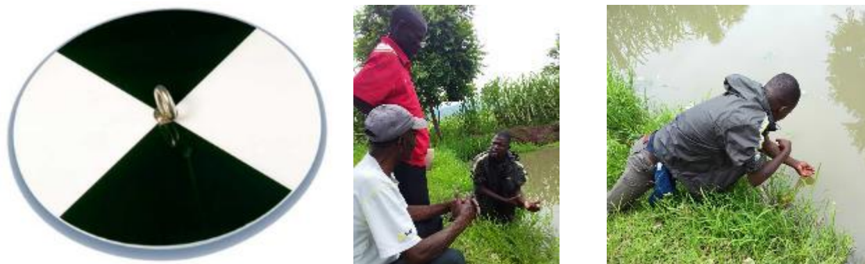
Figure 8: Secchi disk (left), aquaculture specialist demonstrating arm test (centre and right)
