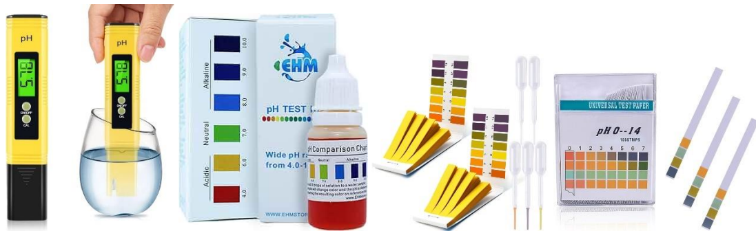
Figure 6 Different methods of measuring pond soil and water pH on your farm
