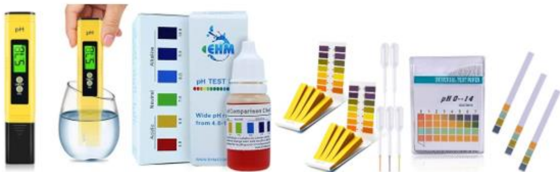
Figure 4 Different methods of measuring pond soil and water pH on your farm
