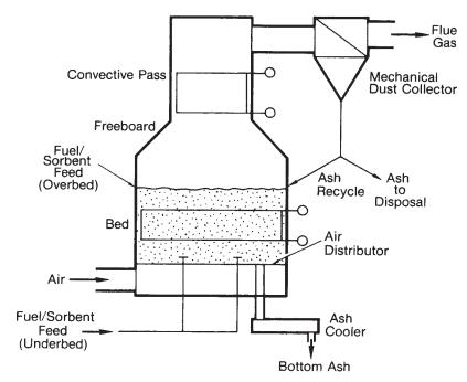
Figure 7-7. Fluidized Bed Boiler (Reproduced with the permission of Ahlstom Power, Inc., Windsor, CT from Combustion Fossil Power (Copyright 1991))
