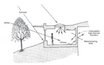
Figure 13-10. Energy conservation through the use of overhangs.
