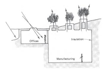
Figure 13-8. Recommended insulation placement
