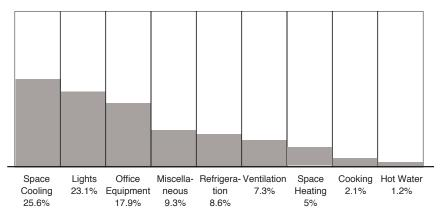
Figure 1-4 Commercial Electric Use 1999 (end-use basis) Source - U.S. Department of Energy EIA (2005)
