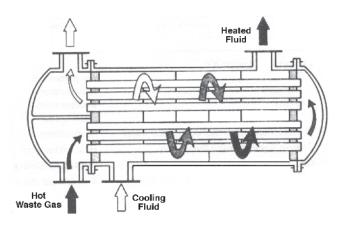
Figure 8-8. Convective-type recuperator. (From [7], Courtesy of the U.S. Department of Commerce.)
