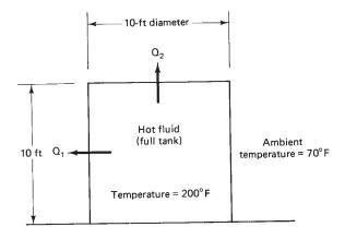
Figure 11-2. Tank storage of hot fluid.
