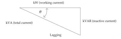
$\theta$  = phase angle = measure of net amount of inductive reactance in circuit  $\cos \theta$  = PF = ratio of *real power* to *apparent power*
