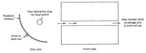
Figure 13-6. Parabolic trough solar collector
