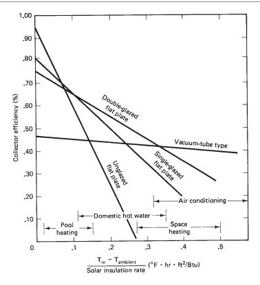
Figure 13-5. Typical flat-plate collector efficiencies
