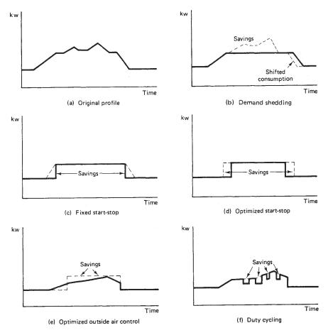
Figure 9-2. EMCS control techniques. (From Dick Foley, "Reducing Waste Energy with Load Controls," *Industrial Engineering*, July 1979, p. 24. Extracted with permission from Institute of Industrial Engineers, Inc., 25 Technology Park/Atlanta, Norcross, Ga., 30092, ©1979.)
