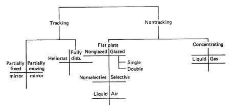
Figure 13-2. Types of solar collectors.
