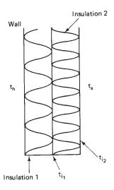
Figure 11-3. Insulation system.
