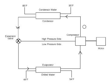
Figure 6-4. Diagram of a typical chiller.
