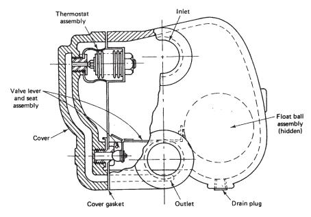
Figure 8-3. Float and thermostat steam trap (Courtesy of Armstrong Machine Works)
