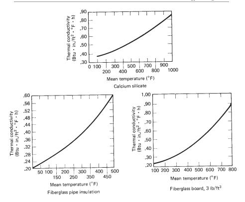
Figure 11-1. Thermal conductivities at varying temperatures.
