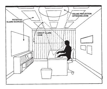
Veiling reflections commonly occur when the light source is directly above and in front of the viewer, in the "offending zone."
