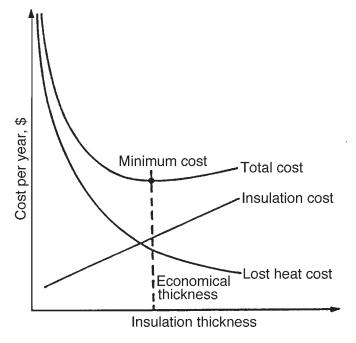
Figure 11-4. Illustration of the economic thickness of insulation.
