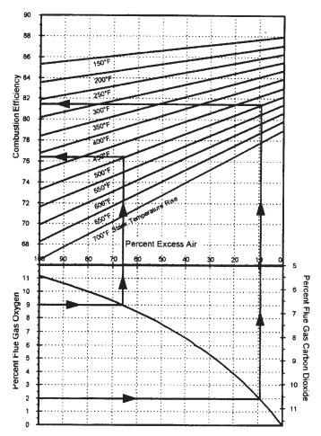
Figure 7-11. Example of a combustion efficiency curve and its use, (From S.A. Parker; R.B. Scollon; and R.D. Smith, "Boilers and Fired Systems," Chapter 5 in *Energy Management Handbook, Fourth Edition*, Wayne C. Turner, Senior Editor, Fairmont Press, 2001, reproduced with permission).
