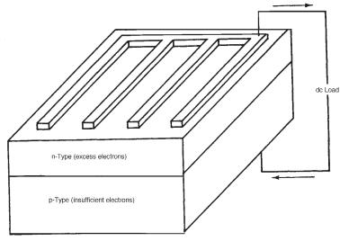
Figure 13-12. Typical photovoltaic cell
