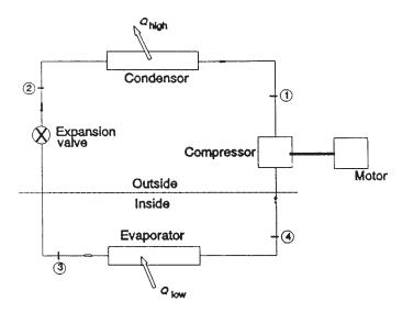
Figure 6-3. Vapor compression refrigeration cycle.
