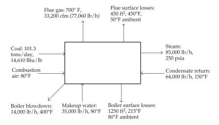
Figure 7-9. Mass Balance for a Typical Boiler
