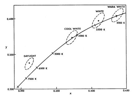
Figure 5-1. Fluorescent Lamp Color Temperatures [ref 1, Figure 5-17]
