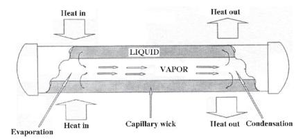
Figure 6-5. Diagram of heat pipe.
