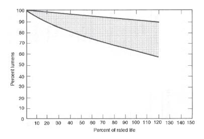
Figure 5-14. Typical lumen maintenance curve for filament lamps. (From General Electric Technical Pamphlet TP-105.
