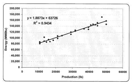
Figure 1-18. Regression Analysis of Food Processing Plant Energy Consumption
