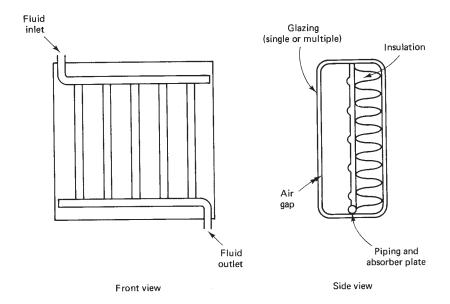
Figure 13-3. Flat-plate solar collector.
