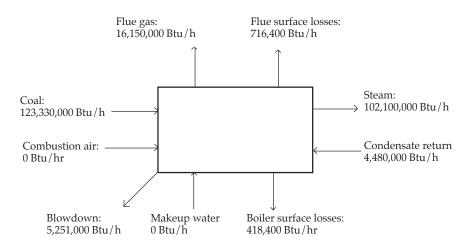
Figure 7-10. Heat Balance for Boiler of Figure 7-9
