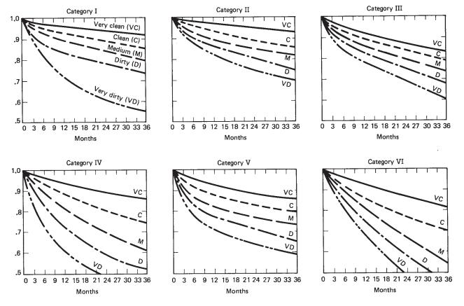
Figure 5-11. Luminaire Dirt Depreciation Factors
