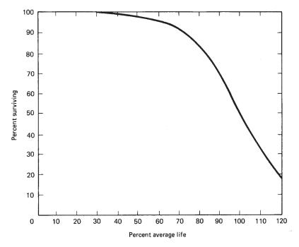
Figure 5-16. Typical mortality curve for fluorescent lamps. (From General Electric Technical Pamphlet TP-105.
