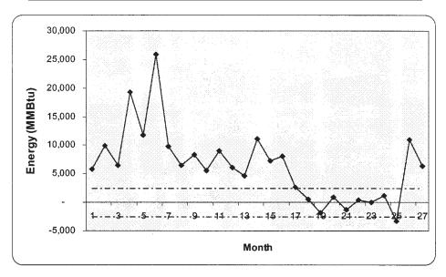
Figure 1-23. Control Chart for Production Example
