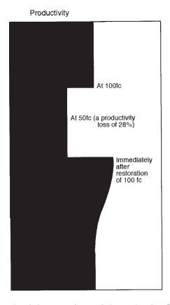
Figure 5-22. Productivity Loss from Light Reduction [ref 6, Figure 2]
