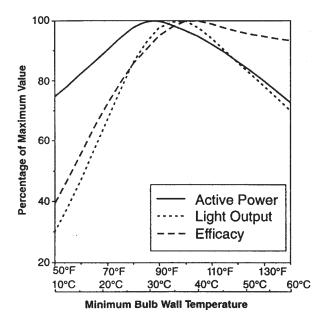
Figure 5-10. Lamp Performance vs. Temperature
