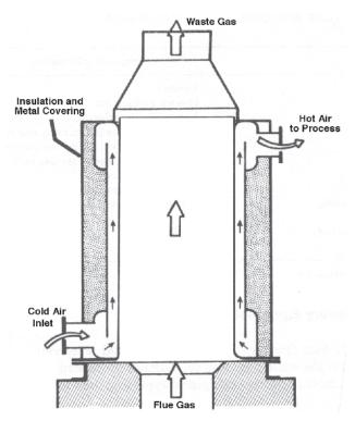
Figure 8-7. Radiation recuperator. (From [7]. Courtesy of the U.S. Department of Commerce.)
