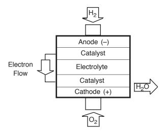
Figure 14-1. Functional Operation of a Fuel Cell
