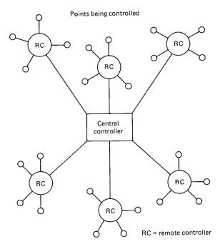
Figure 9-4. Distributed control EMCS star network.
