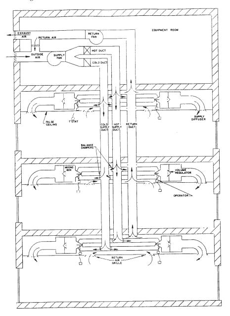
Figure 6-1. Dual-duct HVAC system.
