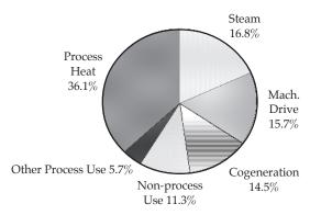
Figure 1-5 Industrial Energy Use 2002 (end-use basis) Source - U.S. Department of Energy EIA (2005)
