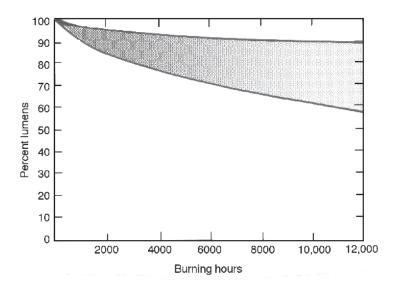
Figure 5-13. Typical lumen maintenance curve for fluorescent lamps. (From General Electric Technical Pamphlet TP-105.
