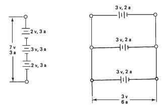
Figure 13-13. Photovoltaic hookups
