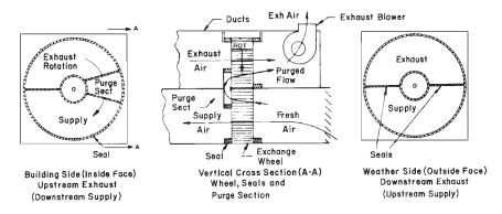
Figure 8-10. Heat wheel with purge section. (From [7], Courtesy of the U.S. Department of Commerce.)
