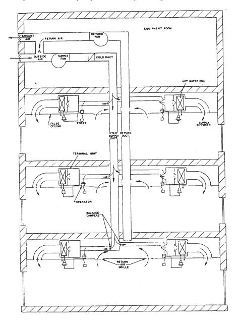
Figure 6-2. Terminal reheat HVAC system.
