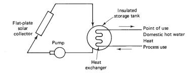
Figure 13-4. Typical flat-plate solar collector application.
