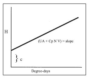
Figure 1-16. Relationship between degree-days and heat load.
