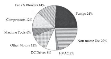
Figure 1-6 Industrial Electricity Use (end-use basis) Source - Federal Energy Management Agency
