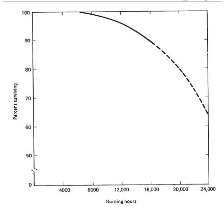
Figure 5-18. Typical mortality curve for HID (mercury vapor) lamps. (From General Electric Technical Pamphlet TP-105.
