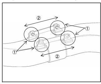
Test fit the exhaust manifold to the cylinder head. Adjustments should be made at the midway insertion section to ensure that the manifold fits correctly.
