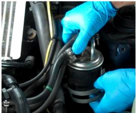
3. Unclip wiring harness clip that attaches to the metal wiring harness bracket.
