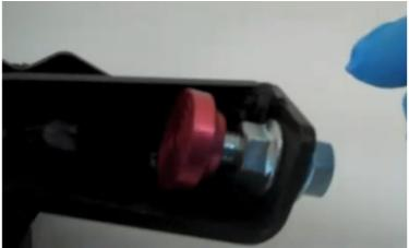
12. Using a 15mm wrench and 5mm hex key, insert hex key into stud and tighten the nut closest to the master cylinder which will extend the stud. Ensure that the other nut is loose. When the pressure cup makes contact with the master cylinder, tighten the nut an additional 1/2 to 1 turn.
