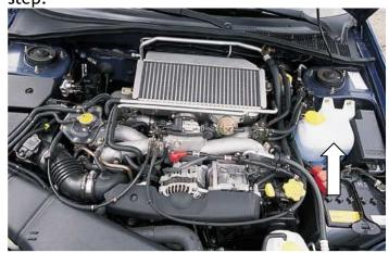
2. Unclip fuel filter and move the filter out of the way. A couple temporary zip ties can be used to hold it out of the way during the install. Later models can skip this step as the fuel filter is not mounted here.
