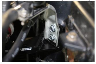
9. Tighten all 4 bolts using a 10mm socket to 15 ft-lbs.
