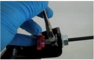
13. Now tighten the other nut to lock the adjustment into place.
