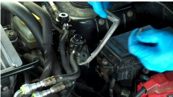
5. Later models have a secondary air injection pump that must be moved out of way to access the bolt for the fuel holder. Remove the 2 bolts on the strut tower, the one bolt towards the battery, the hose on top of pump, and the electrical connection. Then remove from car.
