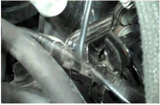
4. Remove fuel filter bracket (earlier models) or fuel line bracket (later models) by removing 2 bolts. These holes will be reused to mount the brace. The wiring harness bracket can be removed and will not be reused.
