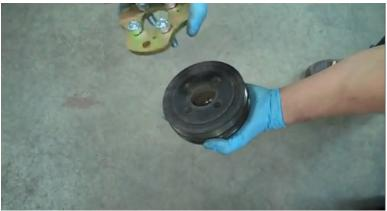
12. If your OEM pulley looks like this, you will install the 4 smaller pins into the GrimmSpeed crank pulley removal tool using an 11mm wrench.
