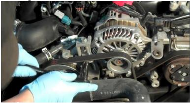
4. Then loosen the tensioning rod with a 12mm socket.
