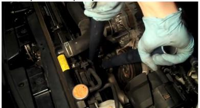
15. Rock the OEM pulley back and forth and pull it out from the engine. Be sure to clean the end of the crank shaft to remove any dirt or debris.
