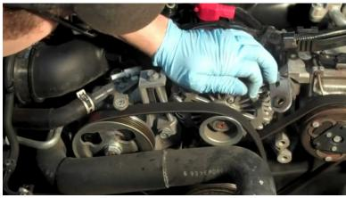
7. Removal of A/C belt for pre-2008 models. 2008+ owners please skip to install step 9. Loosen the A/C idler tension lock nut using a 12mm wrench.
