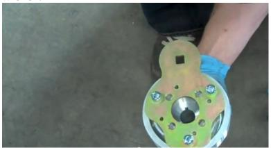
18. Install crank pulley onto crankshaft. WARNING: Be sure to line up the keyway and ensure the pulley is fully seated onto the crankshaft. If you do not, damage can occur to your pulley or crankshaft.
