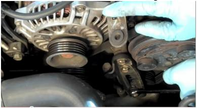
8. Loosen the tensioning rod with a 12mm socket and remove the belt.
