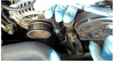
22. Tighten the A/C idler tension lock nut using a 12mm wrench.
