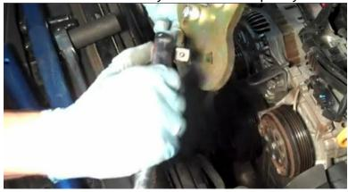
14. Insert a 22mm socket (we've found a deep socket works the best) into the crank pulley bolt. Then insert a breaker bar onto the socket. You will be rotating the crank pulley bolt counter clockwise. Hold the pulley from rotating with the ratchet that is installed on the GrimmSpeed crank pulley removal tool. Loosen the bolt and remove it.
