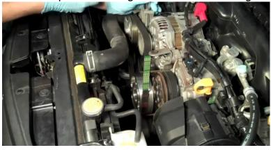
35. Tighten the tensioner lock bolt and the right alternator pivot bolt. Be sure to align the bracket to allow for easy belt cover installation.
