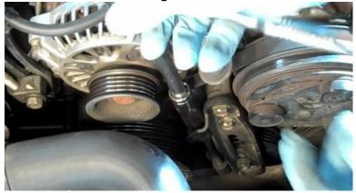
9. Removal of A/C belt for 2008+ models. Pre-2008 owners please skip to install step 14. Because your car does not have a belt tension idler for the A/C compressor, you will need to rotate the engine and feed the belt off of the A/C compressor pulley. Set the parking brake on your car and place the car in neutral. Using a 22mm socket and 1/2" drive ratchet rotate the engine in a clockwise direction.
