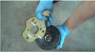
13. Insert a 1/2" drive ratchet or breaker bar into the GrimmSpeed crank pulley removal tool and insert the tool into your OEM crank pulley.
