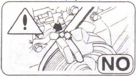
33. Before starting the engine, rotate the crankshaft 2X in the clockwise direction to ensure
