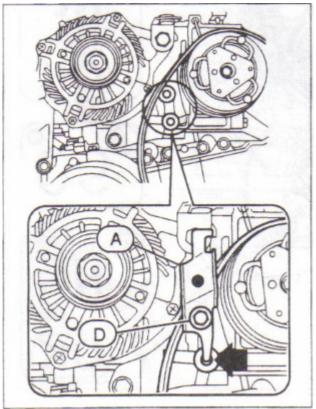
27. Loop the belt around the crank pulley tool as shown.
