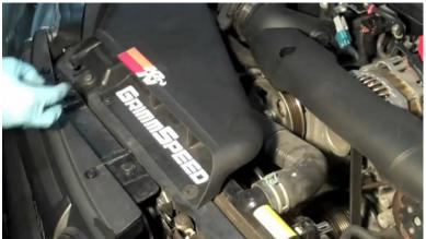
2. Using a 10mm wrench, remove the accessory belt guard. Once the bolt and nut is removed, you can unsnap it. Gently unsnap the 2 snap locations independently and do not
