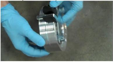
25. Rotate the pulley clockwise so that the tool is approximately 45degrees from the 12 o'clock position.
