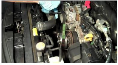
36. Install belt cover and install bolt and nut with a 10mm socket.
