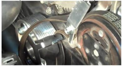
28. Ensure the belt ribs are facing backwards like the image below.
