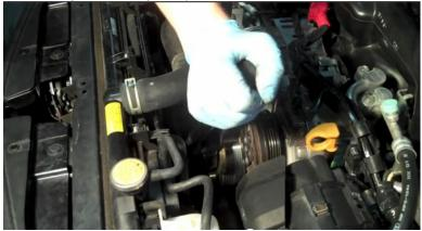
21. Installation of A/C belt for pre-2008 models. 2008+ owners please skip to install step 23. Inspect old belt and replace if worn. Install belt onto crank pulley and A/C pulley. Tighten the tensioning rod using a 12mm socket to the OEM spec.
