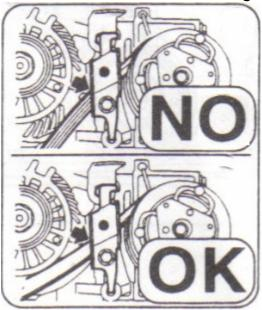
29. Using a 22mm socket, rotate the engine over to feed the belt onto the pulley.
