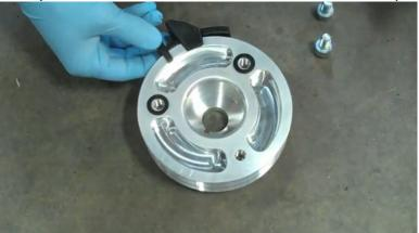
24. Tighten the GrimmSpeed light weight pulley stretch tool onto the pulley as shown with the Gates plastic belt ramp. You will use an 8mm hex wrench.
