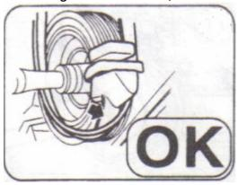
30. Continue rotating the engine to fully place the belt into position. Be careful to not let the belt catch on anything.
