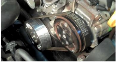
34. Install power steering/alternator belt and tighten the tensioner rod using a 12mm socket.
