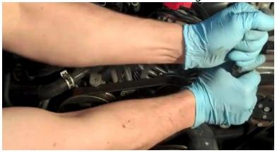
6. Press down on the alternator to relieve the belt tension and remove the belt.
