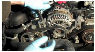
5. You will then need to loosen the right alternator tension bolt with a 12mm socket.
