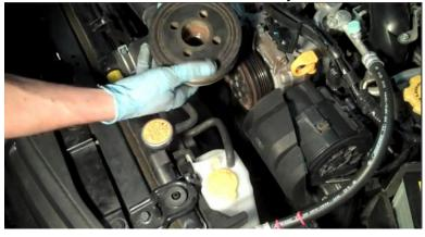
16. You will now be installing the GrimmSpeed crank pulley. Place 3 black nylon washers onto the face of the pulley to protect the finish from the removal tool.
