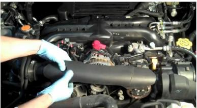
37. Install inlet air duct by reusing the supplied clips. Start engine and verify there the correct belt tension. Congrats, you are done!
