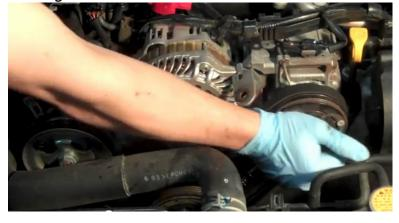
10. While you are rotating the engine by hand, pull on the belt with light tension 2-3" before it contacts the A/C compressor pulley. You will need to rotate the engine 1-2 full revolutions before the belt is fed off.
