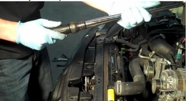
20. Torque crank pulley belt to 94 ft. lbs.
