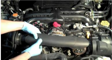
3. Using a 12mm socket, loosen the alternator tension lock bolt.
