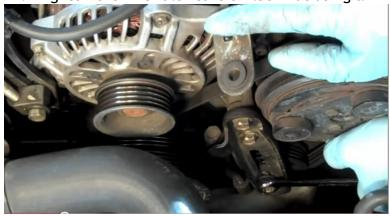
23. Installation of A/C belt for 2008+ models. Pre-2008 owners please skip to install step 34. Your car does not have an A/C tension idler and utilizes a stretch fit belt. You will need the GrimmSpeed light weight pulley stretch tool along with the Gates stretch tool to install this belt. Install the provided nylon washers onto the pulley to protect the finish. Note: Pulley is shown outside of the car for clarification purposes.
