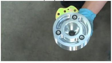
17. Install GrimmSpeed pulley tool and fasten using the 3 supplied fasteners with a 10mm hex wrench.
