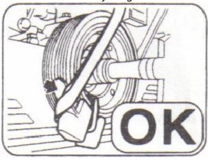
31. Ensure the belt is properly seated in all the grooves.
