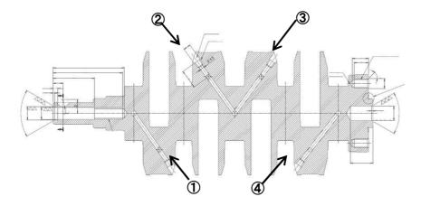
The Crankshaft must be thoroughly cleaned prior to installation. All signs of unwanted debris and residue must be removed from the Crankshaft and the PT 1/16 blind screws (included in the kit).
