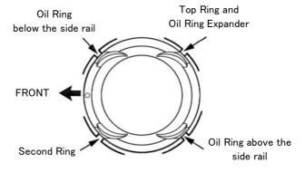
Nosition the clock mark side of the ring up.
