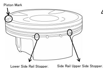
The Oil Ring Side Rail Stopper must be positioned against the raised stopper part of the Piston (as shown on the left).
