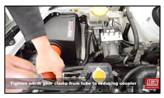
22. You may need to adjust the rotation of the intake tube slightly, to ensure that it's not rubbing on other hoses.
