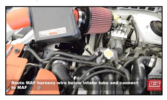
18. Get the heat shield assembly into position and then push the intake tube down towards the fender to ensure that you have plenty of slack in the MAF harness wire. At this point, go ahead and use the rubber grommet and heat shield slot from earlier to safely secure the MAF wire.
