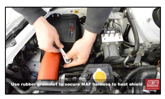
20. Reinstall the two 10mm nuts to secure the heat shield to the vehicle using a 10mm socket.
