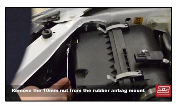
6. Using a 10mm socket and extension, remove the 10mm bolt that secures the airbox to the frame rail. To locate this, look straight down at the frame rail from above the airbox.
