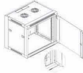
Install front door.
