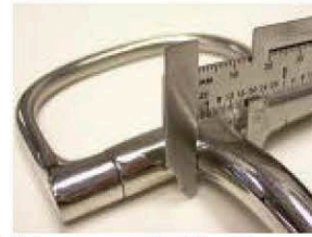
Diameter of bit is measured at the rings or cheeks of the mouthpiece
