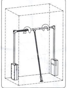
5. Adjust the bar to the suitable postion and revolve it till tighten point according to direction of photo showed. Then fasten the hexagan head screw
