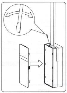
2. After installation, align and flatten the decorative cover. Insert a slotted screwdriver into the removal hole and pry it forward to remove the decorative cover.
