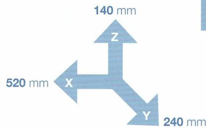
**TRAPANO-FRESA CON ASSI X-Y INTERPOLATI IN CONTINUO E CICLI PROGRAMMABILI DA CN**
