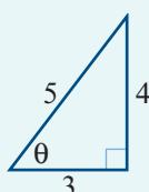
$$\begin{aligned}\text{b } \tan(2\theta) &= \frac{2\tan \theta}{1 - \tan^2 \theta} \\ &= \frac{2 \times \frac{4}{3}}{1 - \frac{16}{9}} \\ &= \frac{2 \times 4 \times 3}{9 - 16} \\ &= -\frac{24}{7}\end{aligned}$$
