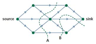
**Cut capacity:** the sum of all capacities of the edges that the cut passes through, taking into account the direction of flow
