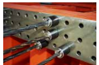
Prestressing wires fixed with anchor grips on the reaction beams
