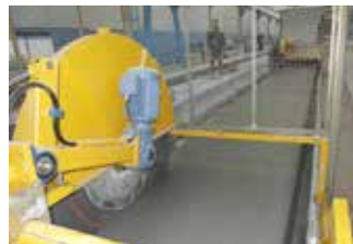
Fresh concrete saw
