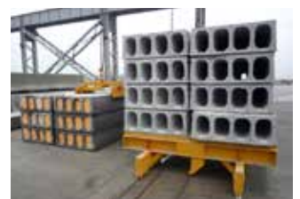
Double element transport wagons
