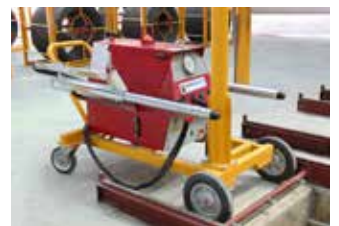
Wire stressing machine holder trolley for movability and to support the stressing jack during the steel wire stressing (Optional)
