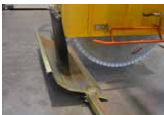
Casing for cutting water collecting
