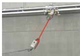
Sliding trolley with 3 axes movement
