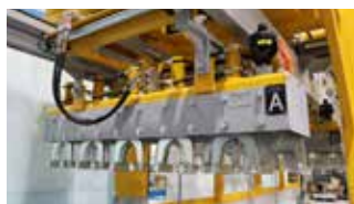
Lifting clamps actioned hydraulically
