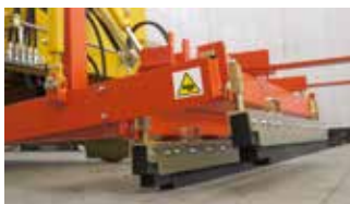
Replaceable squeegee for water collecting
