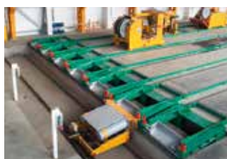
Reaction beams (tensioning and detensioning side)
