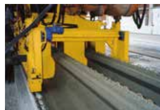
Inverted double T slabs
