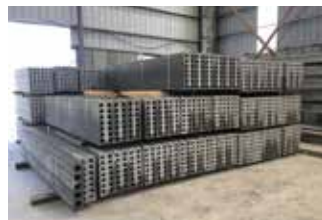
Storage of partition wall panels
