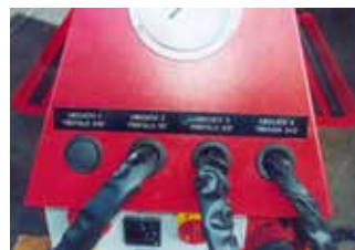
Each stressing jack has its own dedicated hydraulic circuit
