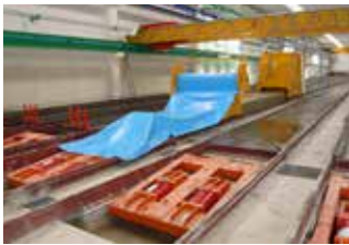
Coiler holding trolley behind the casting machine
