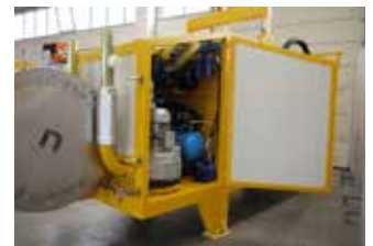
Vacuum assembly with sound insulated inspection panel
