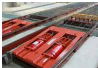
Reaction beam (detensioning side)
