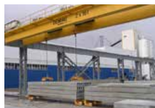
Concrete element transport line
