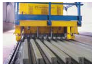
Inverted T beams
