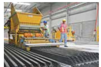
Inverted T beams
