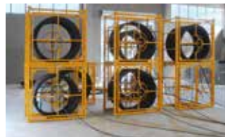
Stackable decoilers for strands or 2-3 wires
