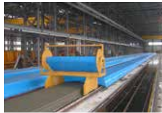
Coiler holding trolley - manual type
