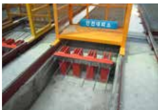
Reaction beam (tensioning side)
