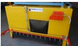
Water tank to apply water to the production bed using drippers, during the cleaning phase
