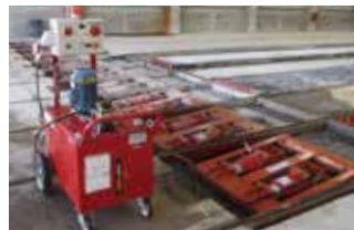
Detensioning pump unit connected to detensioning cylinders
