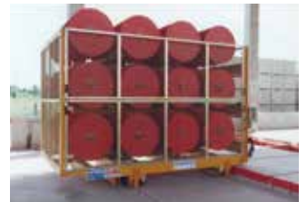
Safety grill protections with side and back panels
