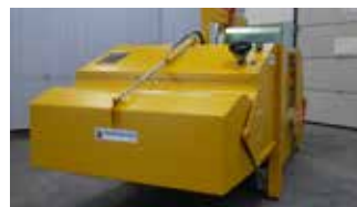
Container for collecting debris and water with hydraulically powered emptying
