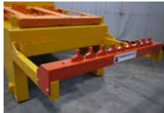
The anchor and the wire spacer in their positions on the trolley
