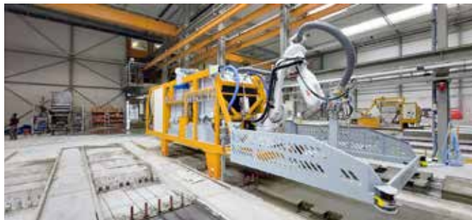
Automatic concrete aspirator
