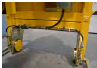
Washing device for cutted element
