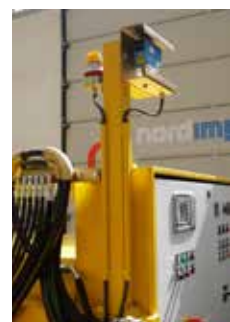
Laser device for automatic movement control
