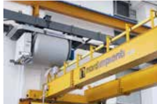
Fly bucket with the concrete distributor
