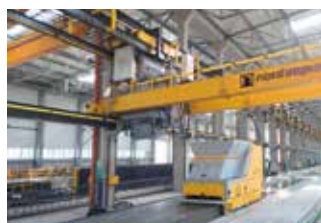
Fly bucket filling the concrete distributor
