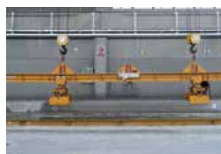
Double lifting hook for long lifting beams
