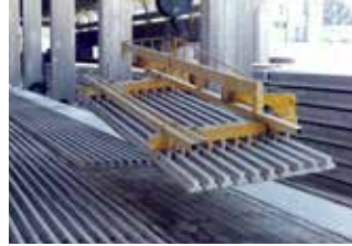
Mechanical lifting beam for inverted T beams
