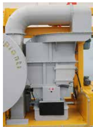
Container for collecting debris and water with hydraulically powered emptying
