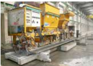
Casting machine being transferred from one bed to another without the need of an overhead crane
