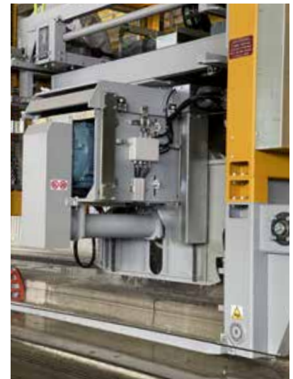
Double protection shield (one mobile and one fixed) for protection when the cutting blade is in operation
