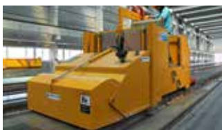
Multifunction bed cleaner with rotating brush
