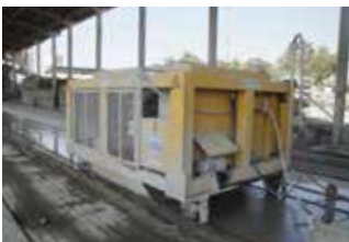
Milling machine for concrete beds
