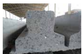
Element with uneven lower surface produced on a worn bed
