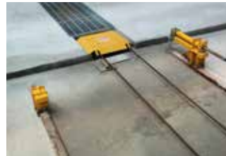
Buffer cylinder with safety protections
