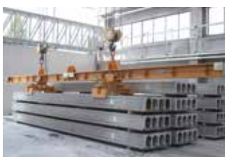
Mechanical lifting beam for hollow core slabs
