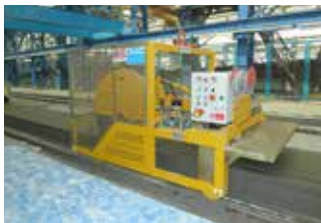
Fresh concrete saw
