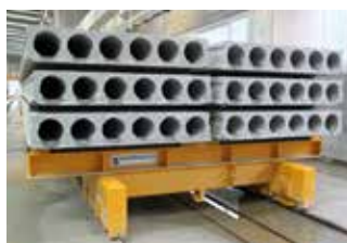
Double element transport wagons
