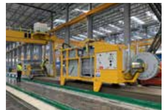
Concrete aspirator working behind the casting machine
