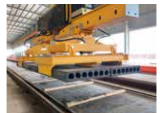
Hydraulic lifting clamps for wall panels
