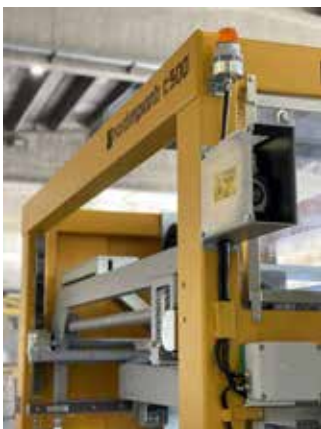
Laser device for automatic movement control
