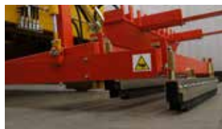
Replaceable squeegee to spread the detaching oil
