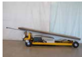
Trolley in the transport position of the wall panel
