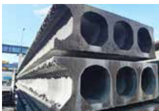
Hollow core slabs longitudinally cut by fresh concrete saw
