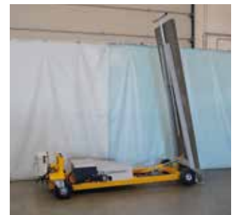
Trolley in the mounting position of the wall panel
