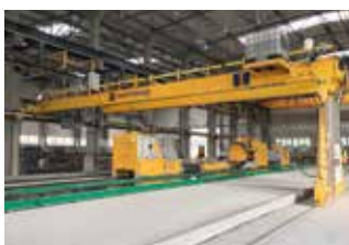
Half gantry concrete distributor
