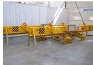
Leg supports when arm is not in use
