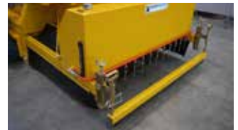
Detaching oil sprayer
