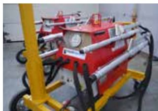
Wire stressing machine with 4 stressing jacks each with 600 mm strokes
