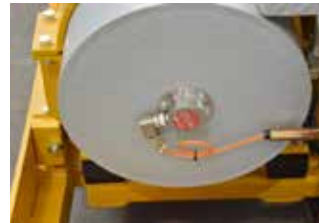
Load cell installed on the stressing cylinders
