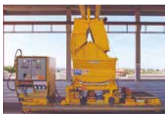
Concrete discharge into the hopper of the casting machine
