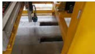
Inkjet head for during the element marking phase
