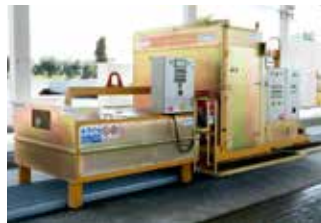
T beam marking machine connected with automatic cutting saw
