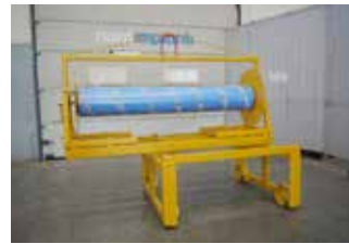
The trolley allows the coiler to be shifted to one side when another machine needs to pass on an adjacent production bed
