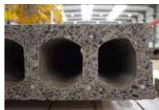
Excellent concrete compaction and steel wire bonding
