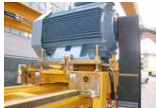
Electric motor and toothed drive belt to rotate the cutting blade
