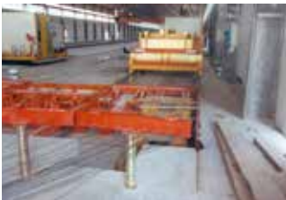
Double wire drawing trolley
