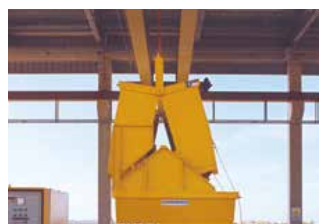
The discharge door is activated mechanically by engaging the steel triangles situated on both sides of the casting machine's hopper
