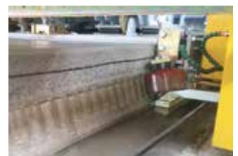
Para-seismic side indenting device (Optional)
