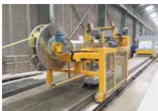
Surface grooves machine which follow the casting machine
