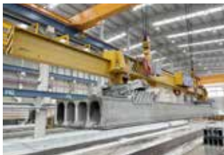
Telescopic lifting beam for hollow core slab
