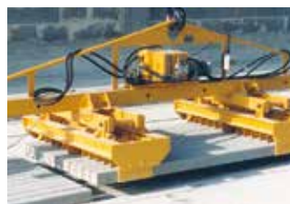
Hydraulic lifting clamps for posts
