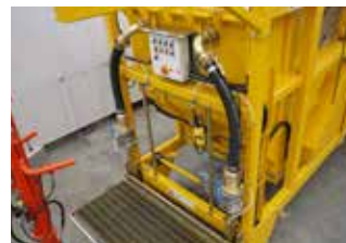
Side vacuum pipes for rail cleaning (Optional)
