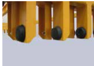
Rubber grips to avoid damage to the elements during lifting
