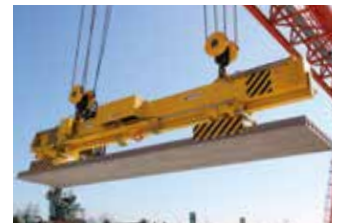
Double lifting hook
