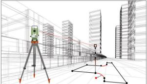
This program facilitates the easy stake out or checking the lines for buildings, sections of road, simple excavations, etc. A reference line can be defined by referencing a known base line. The reference line can be offset either longitudinally, in parallel or vertically to the base line, or be rotated around the first base point as required.
