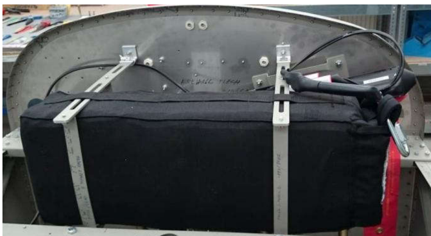
Figure 7-20 AEPS canopy container with packed chute
