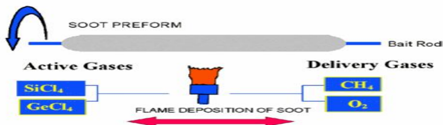
Figure (1) Laydown FOR (OVD)
