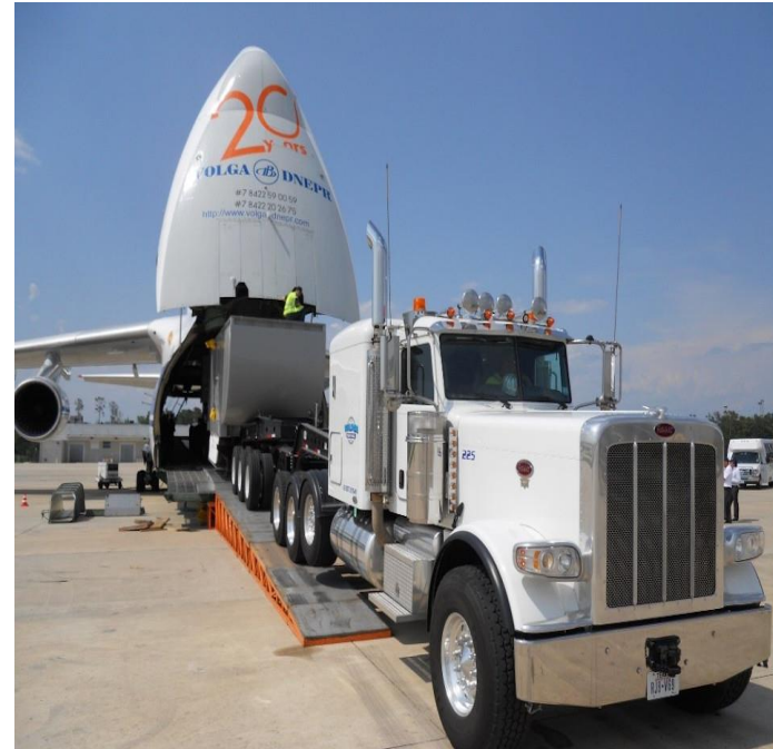
Loading TM2500+ for Air Transport
