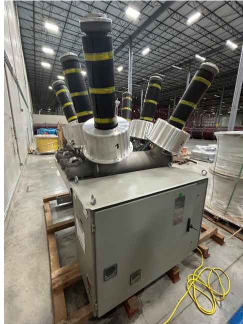
Full unit: tank and low-voltage control cabinet
