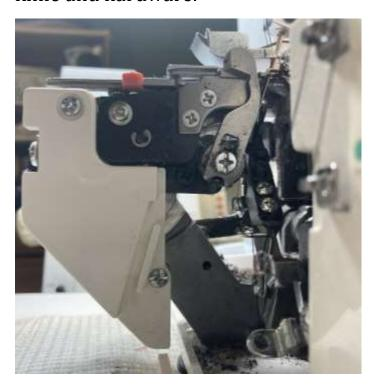
3.8 Thread through the thread guide on the lower looper arm from
