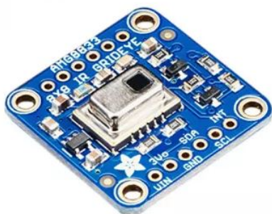
Figure 4.4: Figure depicting the Adafruit AMG8833 device[12]
