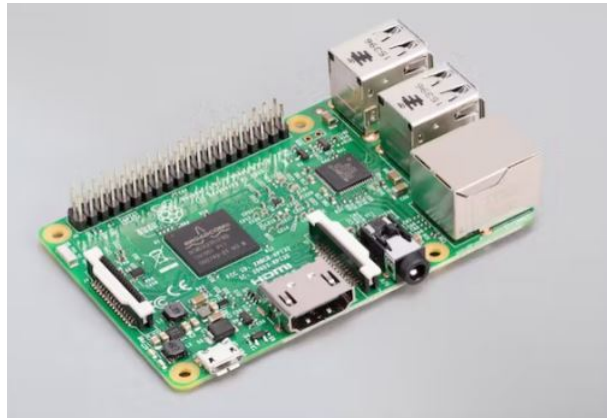
Figure 4.2: Figure depicting the Raspberry Pi 3B [10]
