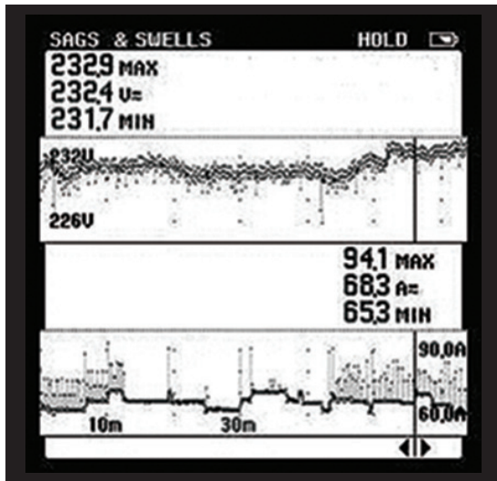
A power quality meter reading: the voltage and amperage levels demonstrate dirty power.
