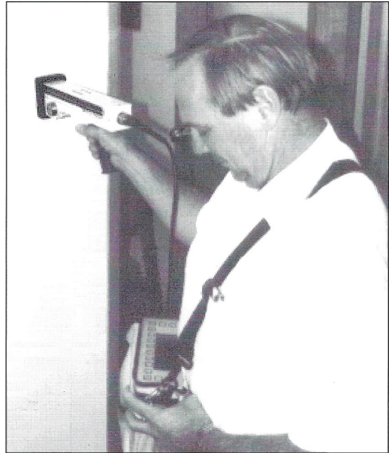
Steven Gehrig checks the readings on an XRF, a device used to measure the amount of lead, if any, on painted surfaces. Gehrig is a facilities inspection specialist with PWC San Diego
