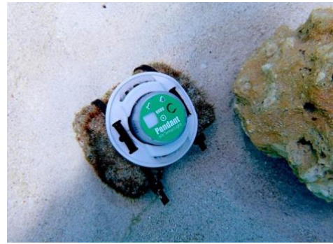
Figure 11 HOBO Light and Temperature Logger in use. Photographer: Jente van Langerak.
