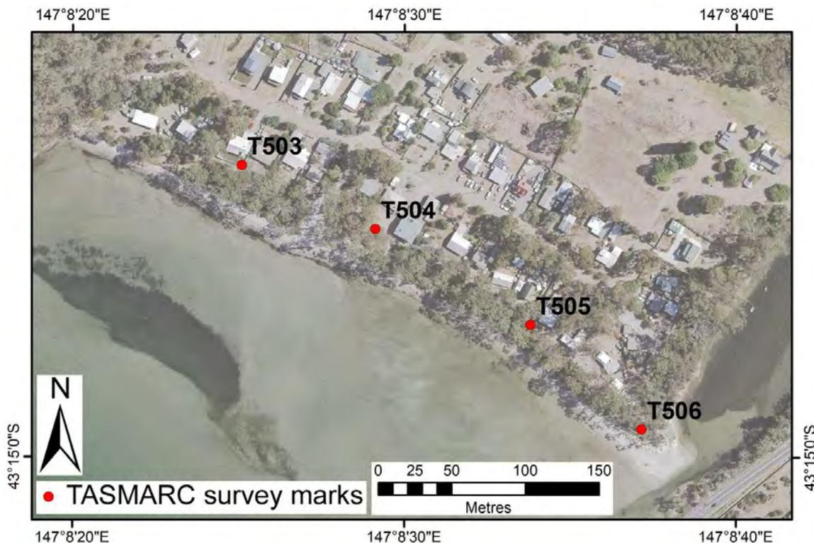
**Figure 35: TASMARC survey mark positions at Garden Island Sands Beach.** Each survey marker is a treated pine post embedded securely in the ground with a stainless-steel screw in the top of the post indicating the precise surveyed marker position. The survey transects extend seawards from the marks, normal (perpendicular) to the shoreline. Background image is the 19<sup>th</sup> of December 2015 air photo (© NRE).
