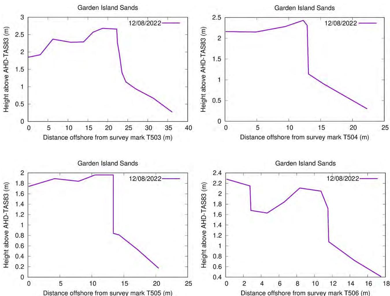
**Figure 17: The first TASMARC profiles surveyed from the 4 survey markers at Garden Island Sands Beach, on 12<sup>th</sup> August 2022.** Survey plots prepared by Nick Bowden; scales are in metres. Note that the vertical scale is exaggerated compared to the horizontal scale, which makes all landform features appear steeper and higher than they really are (albeit the vertical erosion faces are indeed as steep as they appear, but their height relative to the horizontal scale is exaggerated).
