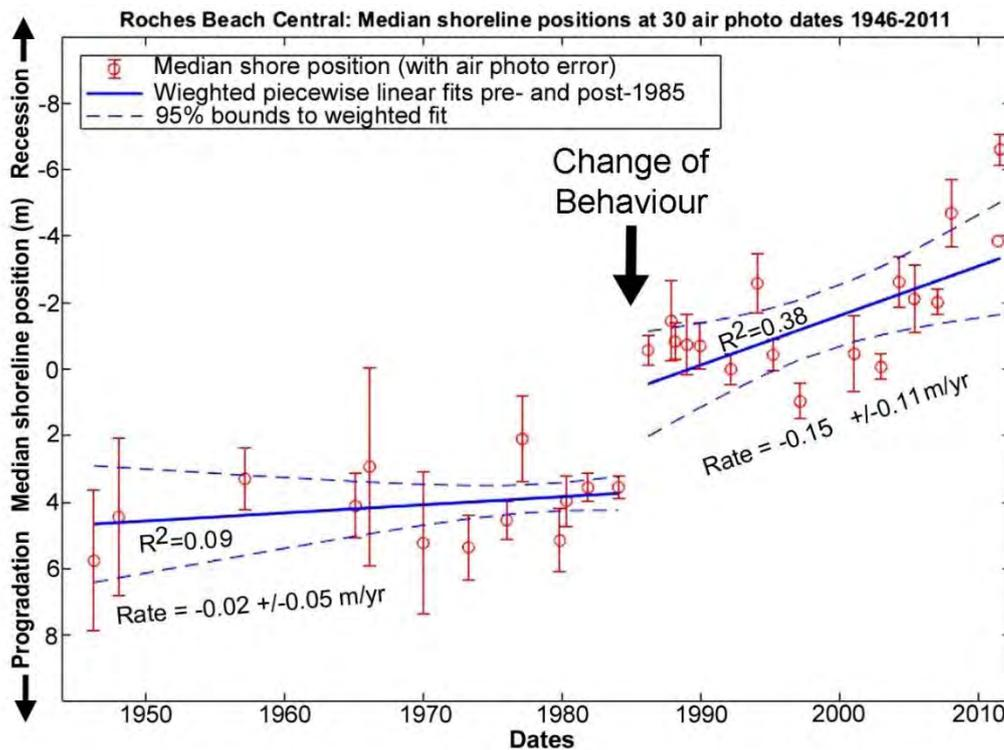
**Figure 34: Shoreline history for Roches Beach central section** (transects 13780 – 13801 except 13798). Median shoreline position across all used transects at each of 30 air photo dates (1946-2011), showing air photo position error bars at each date. Piecewise linear fits around 1985 shown weighted by error margin, with 95% bounds to weighted fit indicated.
