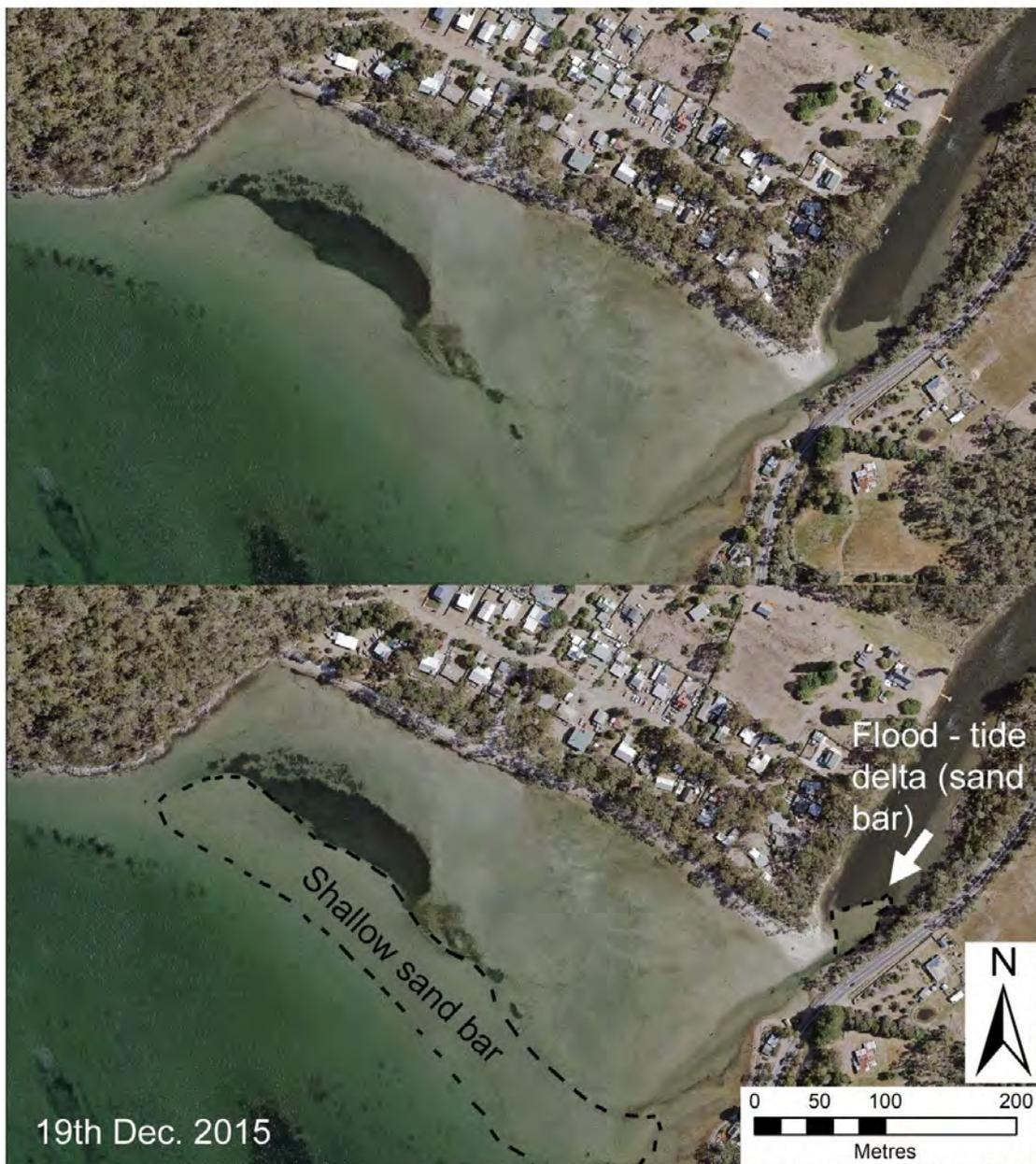
**Figure 9: Air photo of Garden Island Sands showing shallow sub-tidal sand bar features.** Original photo dated 19<sup>th</sup> Dec. 2015 (top) and annotated version (bottom) showing ephemeral sandy flood-tide delta in estuarine lagoon and shore-parallel shallow offshore sand bar encroaching landwards over the margins of a large seagrass bed. Air photo © NRE
