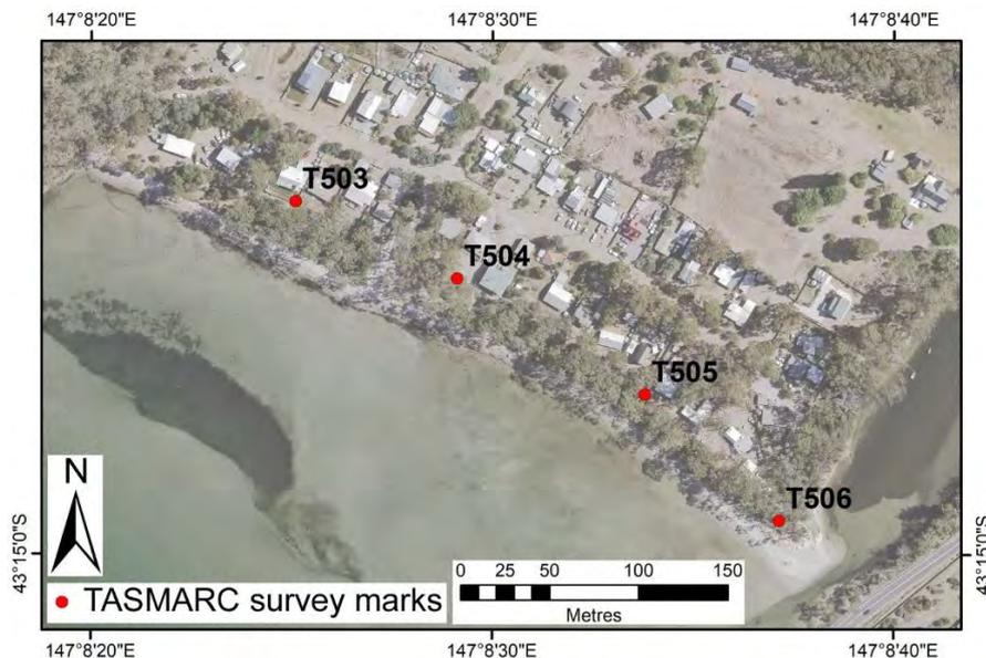
**Figure 16: TASMARC survey mark positions at Garden Island Sands Beach.** Each survey marker is a treated pine post embedded securely in the ground with a stainless-steel screw in the top of the post indicating the precise surveyed marker position. The survey transects extend seawards from the marks, normal (perpendicular) to the shoreline. Background image is the 19<sup>th</sup> of December 2015 air photo (© NRE). For larger version of this figure see Appendix 4.
