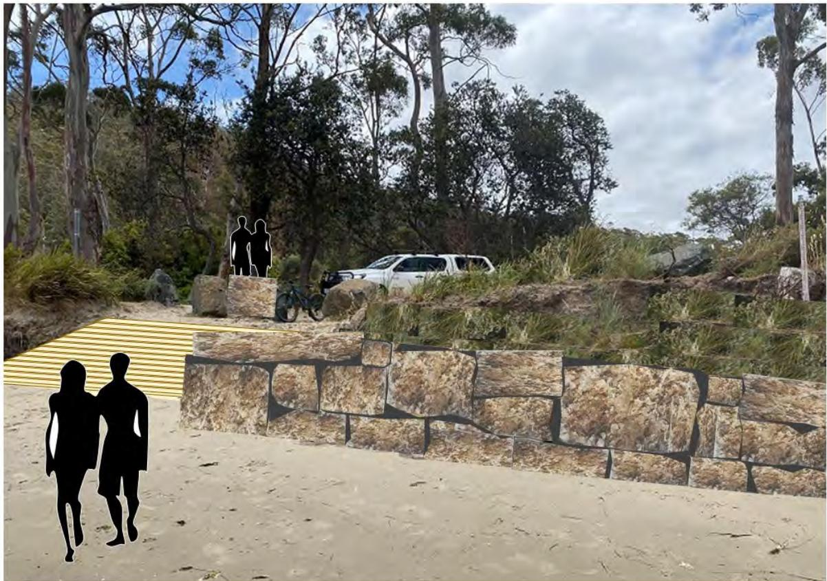
Figure 13. A schematic image of part of the proposed timber access and part of the Stage 1 seawall.
