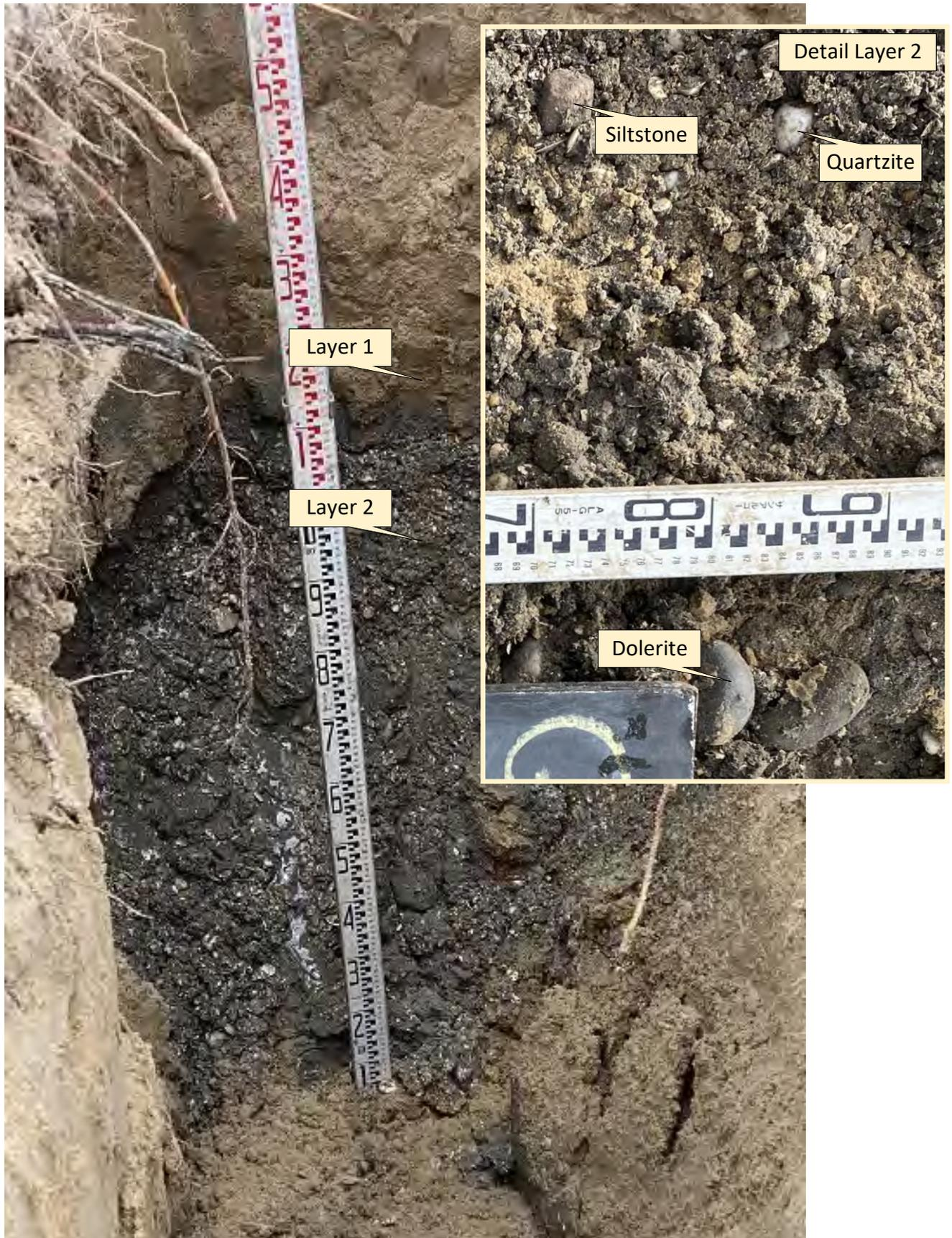
Plate 4 Layers 1 and 2 sand in test pit B. The detail shows types of gravel present in Layer 2. Layers 1 and 2 materials are reasonably typical of materials in all six test pits, and by inference, beneath the full length of the beach. The large numbers on the scale are decimetres.
