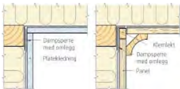
Klemmeprinsipper for dampsperre
