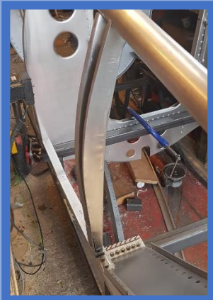
Starboard cockpit framework - including upper and lower longerons.
