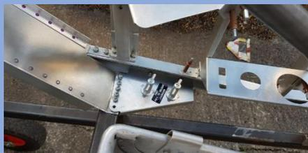
**2** Both toggles fitted to the bracket – right-hand side cockpit.
