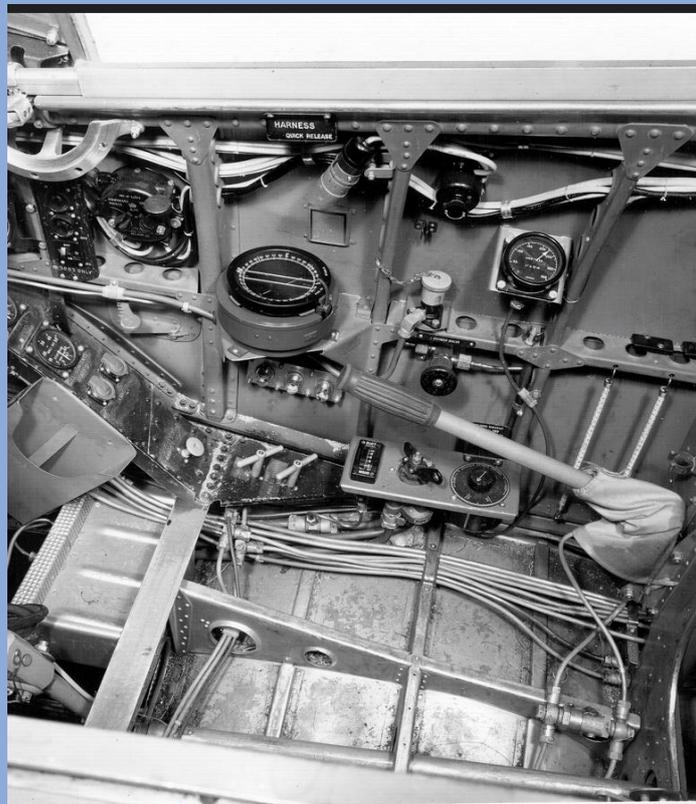
**3** Starboard side cockpit – seat removed.
